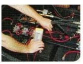
**Test #1:** Touch black wire of voltmeter to car chassis to ground. Touch red wire of voltmeter to +PWR post on Street Charger. Meter should read 12 – 14 volts.
